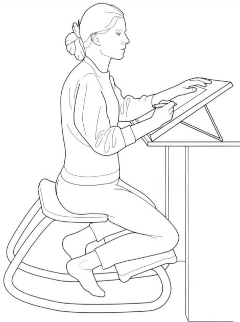
Figure 4.15 The original Norwegian kneeling chair, designed by Opsvik, provides an angle of approximately 135° between spine and thigh, retains the lumbar curve and allows much of the weight to rest on the shins (after Journal of Bodywork and Movement Therapies 4(3):162).
